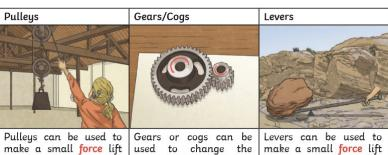
Pulleys can be used to make a small force lift a heavier load. The more wheels in a pulley, the less force is needed to lift a weight. Gears or cogs can be used to change the speed, force or direction of a motion. When two gears are connected, they always turn in the opposite direction to each other.
